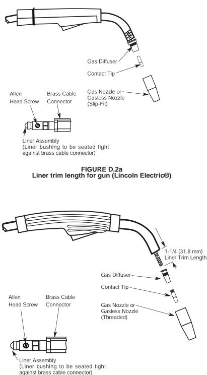
**FIGURE D.2b** Liner trim length for gun (Magnum<sup>™</sup> 100L)
